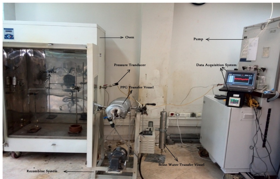
Fig. 2. The experimental set up for retention experiments.
