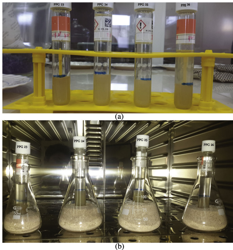
Figure 4. Swelled PPGs: (a) before aging and at room temperature; (b) after aging for 120 days, at 145 °C. Blue line shows the volume of swelled PPGs at room temperature. It can be seen that aging process at high temperature causes the PPGs to undergo syneresis. PPGs 23–26 showed partial syneresis, lost less than 25 % of original volume, and were considered to pass the test.
