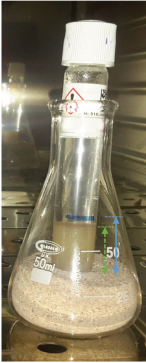
Fig. 8. Swelling ratio measurement of PPGs in NaCl-salinity of 225,000 ppm and different temperatures. (a) 298 K, (b) 418 K. The solid arrow shows the amount of swelled PPGs at room temperature (298 K). The rise of temperature causes the gel to undergo water expulsion and volume reduction (dotted arrow).
